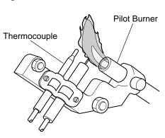
Figure 27 - Incorrect Pilot Flame Pattern
